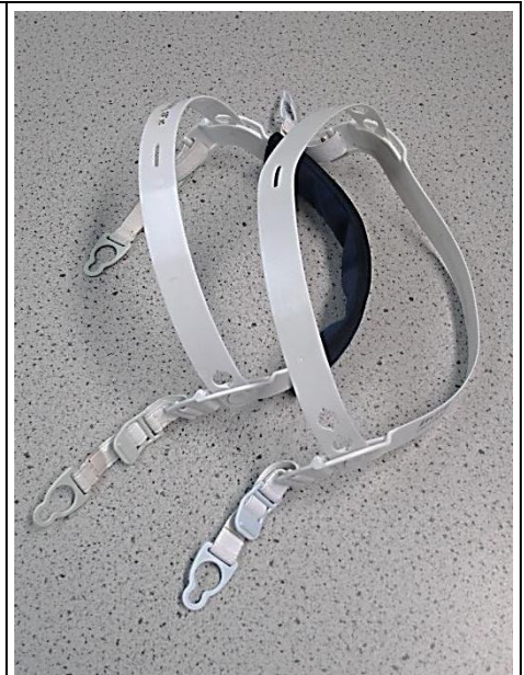
Head harness (Version 1 - with blue padding , Version 2 – with different plastic different elastic and polyester thread)
