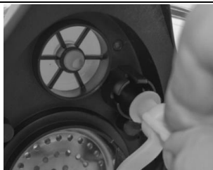
Remove the Sensing Ball from the Sensing Ball socket. Refit the orange plug to the Sensing Ball Socket, pushing it all the way in.
