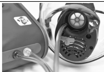
Fit the mask sensing tube to the fit test port (on a TSI PortaCount it is the clear tube).
