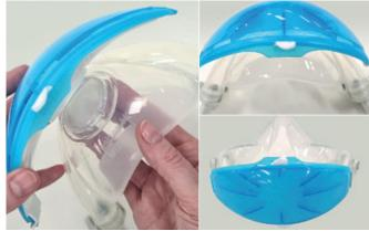
**STEP 4.** Align the assembled case with filter to the mask exhalation cap so the outer case vents are at the bottom of the mask. Click the case onto the exhalation valve seat. NOTE: The exhalation valve cap can remain in place.
