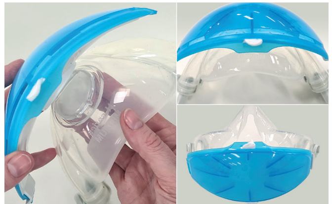
STEP 4. Align the assembled case with filter to the mask exhalation cap so the outer case vents are at the bottom of the mask. Click the case onto the exhalation valve seat. NOTE: The exhalation valve cap can remain in place.
