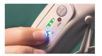
1. Press the on button once to place the respirator in standby mode.
